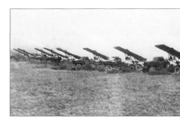
^ A remarkable image of a *Katyusha* formation at the moment of firing. The simplicity of these weapons, coupled with the awesome weight of shot that they could deliver, made them one of the Red Army's most formidable tools. These are firing the 132mm rocket with an 18kg (40lb) warhead.
