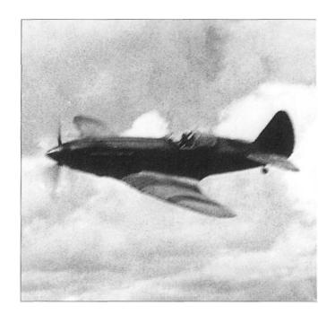
A The Mikoyan-Curevich MiG-3 was an aircraft of very high performance, but one that was difficult to fly. Although originally designed as a high-altitude fighter armed with one 12.7mm and one 7.62mm fixed, forward-firing machine guns in the upper part of the forward fuselage, the MiG-3 could also carry external bomb and rocket loads for ground-attack missions.
