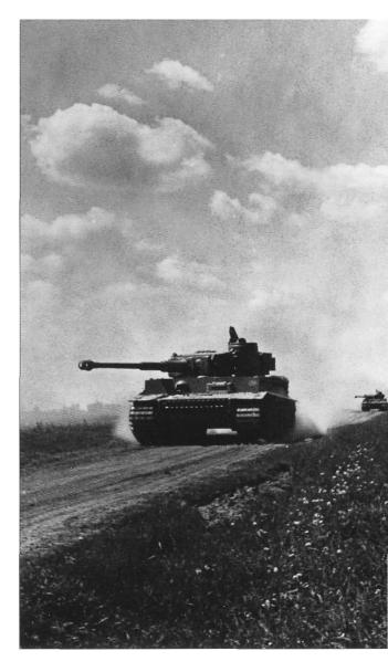
▲ The mighty Tiger entered production in August 1942. Heavily armoured and armed with the formidable KwK 36 88mm gun, it could engage and knock out any Soviet tank before the latter could get within firing range. However, the Tiger was slow and was very expensive to build.
