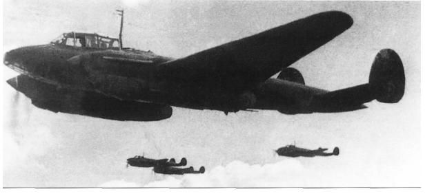
A A flight of Pe-2s proceeds steadily towards its target. The range of the Pe-2, with a bomb load of 10OOkg (2205lb), was 1500km (932 miles), which gave it an unlimited operational capacity over the Kursk salient. The 7.62mm machine gun located in the belly is clearly visible. The nose glazing was intended to increase the accuracy of bomb runs.
