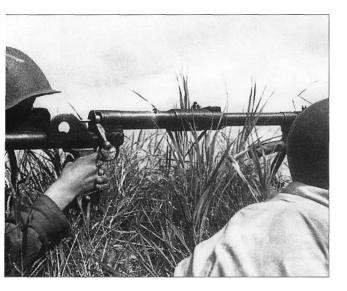
▲ The bolt-action of the single-shot PTRD antitank rifle is clearly shown in this photograph. With a calibre of 14.5mm, the PTRD packed a formidable punch and was much valued as a sniping weapon. Stability was provided by a metal bipod.
