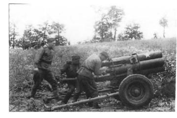
A Turned against its own, this captured German *Nebelwerfer* (literally smokethrower) is speedily reloaded by its Soviet crew in an operation that will take approximately 90 seconds. Each high-explosive rocket weighed some 34kg (75lb). The angle of the tubes would suggest that the target is an armoured vehicle approaching over the crest of the ridge. The white star indicates an earlier "kill" possibly by this unorthodox method of firing.
