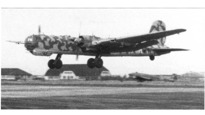
▲ The Heinkel He 177 Greif was a long-range bomber that had a poor combat record. The aircraft was overweight, had structural weaknesses and frequently suffered from engine fires. Around 20 were used during the Stalingrad relief operation.
